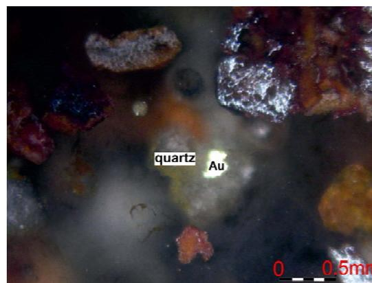
Fig 7. Grain of native gold (Au) included in quartz crystal. Reflected light.
